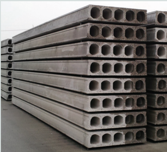
Figure 2. Hollow-core slabs produced by extrusion method.
